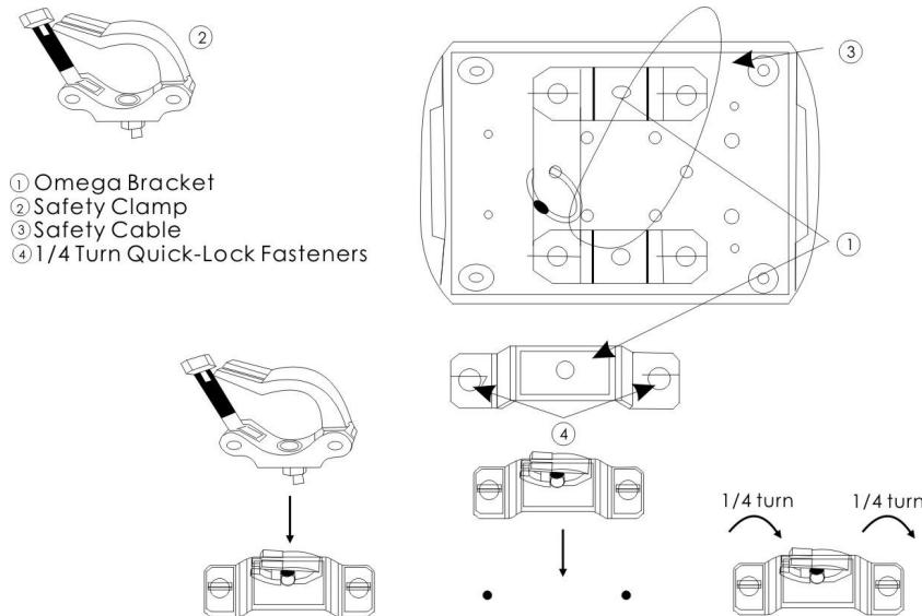
Regardless of the rigging option you choose for your LED moving head, always be sure to secure your fixture with a safety cable. The fixture provides a built-in rigging point for a safety cable on the hanging bracket as illustrated above. Be sure to only use the designated rigging point for the safety cable and never secure a safety cable to a carrying handle.
