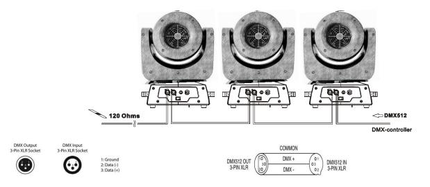
For installations where the DMX cable has to run a long distance or is in an electrically noisy environment, such as in a discotheque, it is recommended to use a DMX terminator. This helps in preventing corruption of the digital control signal by electrical noise. The DMX terminator is simply an XLR plug with a 120  $\Omega$  resistor connected between pins 2 and 3,which is then plugged into the output XLR socket of the last fixture in the chain. Please see illustrations below.
